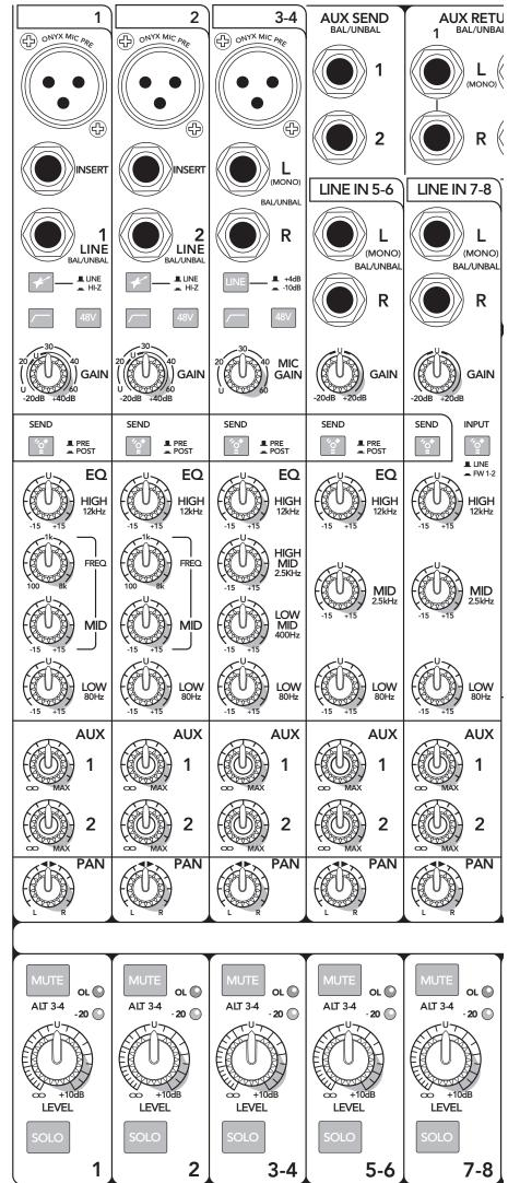
The vertical channel strips look very similar, and have only a few differences between them. Each channel works independently, and just controls the signals plugged into the inputs directly above it.
