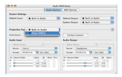
You can also choose it as your default input or output, as well as designate it to be used for system sound output. There are 8 channels of audio input from the Onyx 820i, and 2 channels of audio output to the Onyx 820i.
