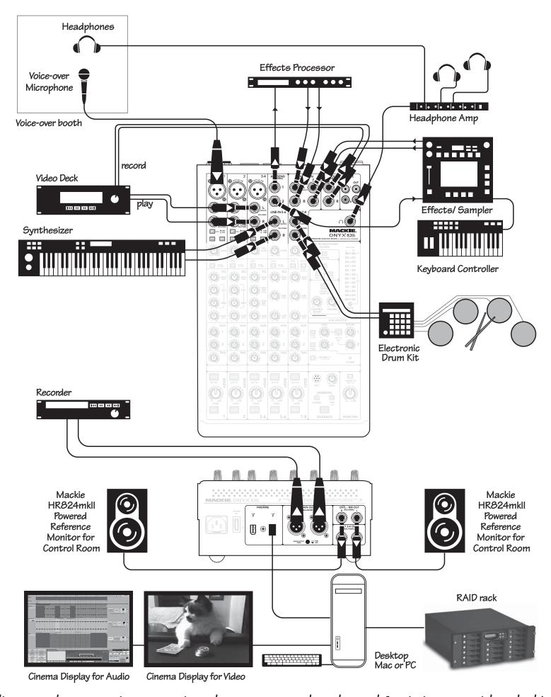
This diagram shows a voice-over microphone connected to channel 1 mic input, a video deck's audio output connected to channels 3/4, with its audio inputs receiving the main mix from the 1/4" outputs. A synthesizer is connected to channel 5/6, and an electronic drum kit connected to channel 7/8.
