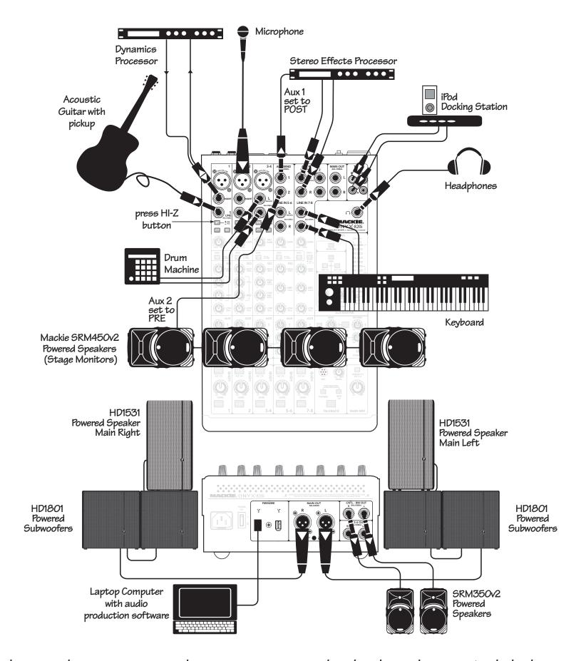
This diagram shows an acoustic-electric guitar connected to the channel 1 input (with the hi-z switch pressed down), a microphone connected to the channel 2 mic input, a drum machine connected to channel 3-4, and a keyboard connected to channel 7-8. Engage the +4dBu/-10dBV switch on channels 3-4 if your drum machine runs at -10 dBV. An iPod® can be used for intermission music.
