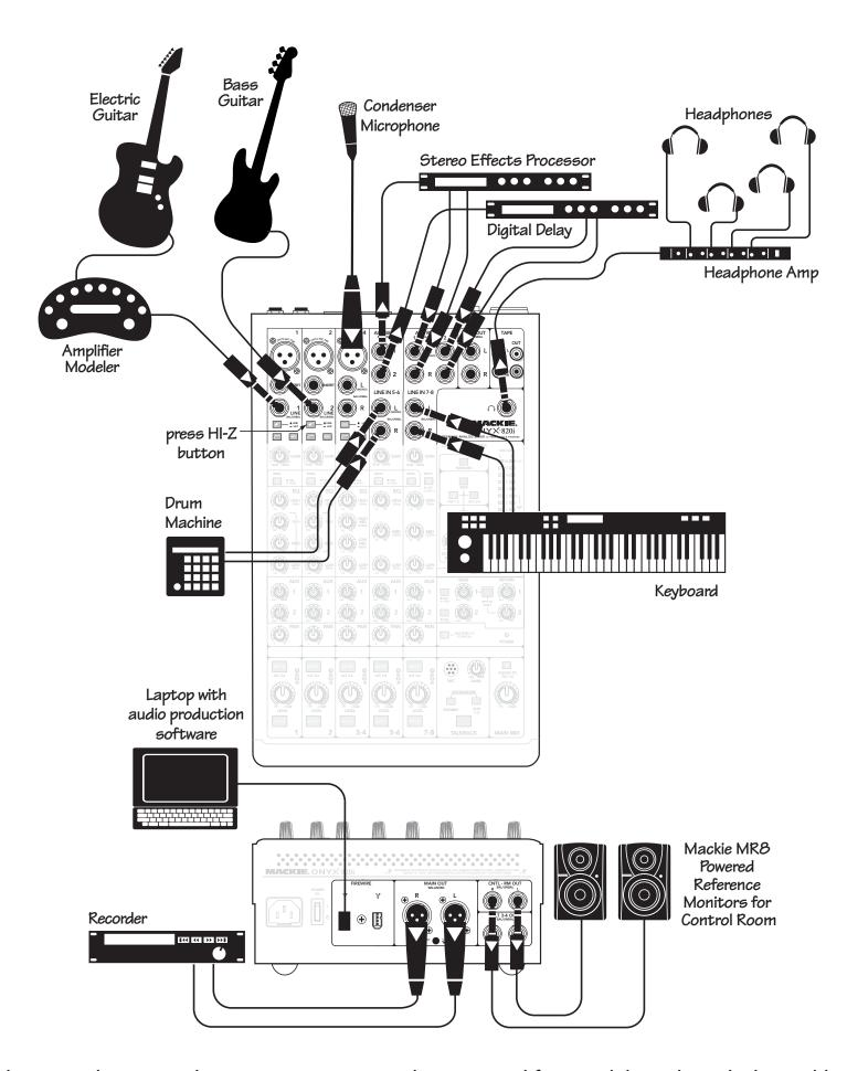
This diagram shows an electric guitar connected to an amplifier modeler, whose balanced line-level output is connected to the channel 1 line input, a bass guitar connected directly to the channel 2 input (with the hi-z switch engaged), a condenser microphone on channel 3/4 with phantom power engaged, a drum machine connected to channel 5/6, and a keyboard connected to channel 7/8. A headphone amplifier allows for multiple headphone use.
